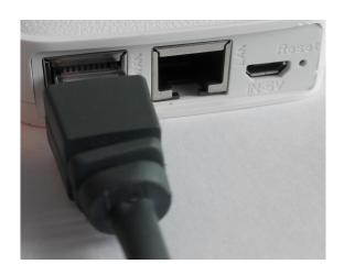
2) Connect the other end of the ethernet cable to an ethernet port on the router given by your internet service provider. An example is shown below.
